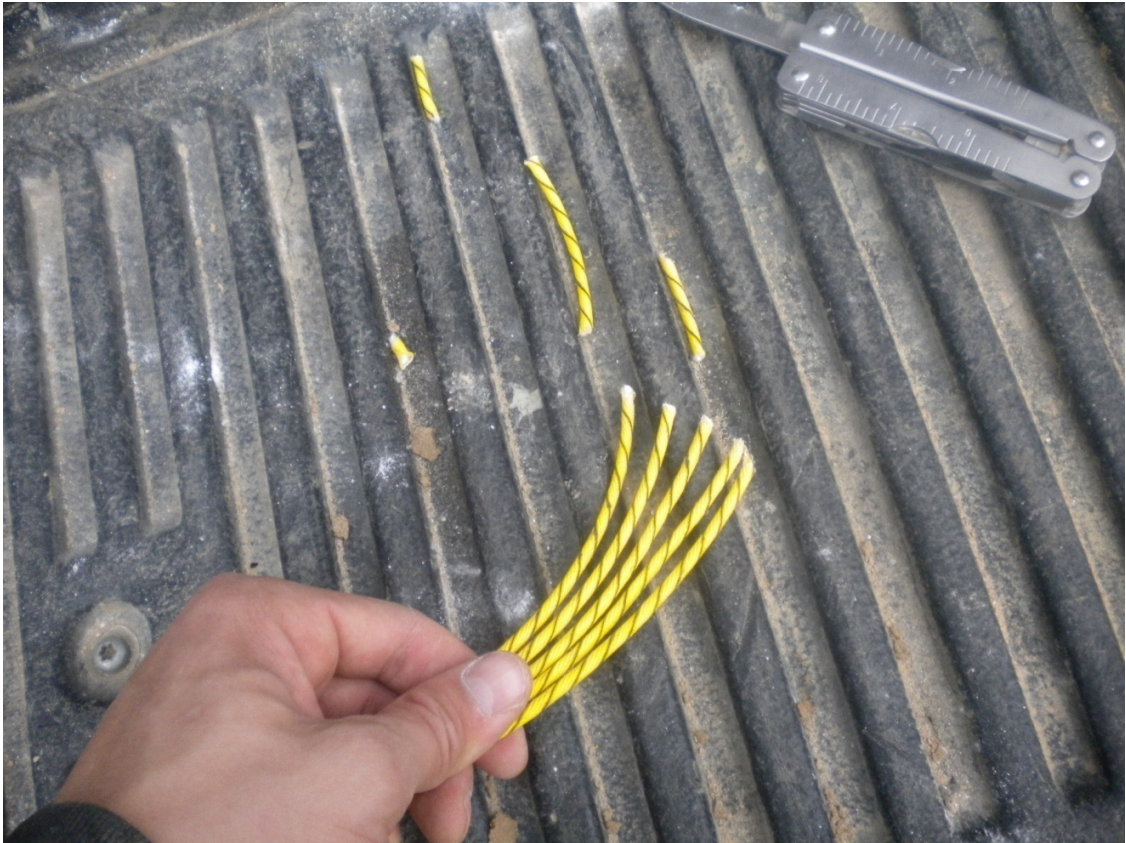
Figure 5.10: The length of each donor cord was measured to ensure that the distance between the detonator connection to the “down-the-hole” cord connection was exactly the same for each hole in the shot. Tips were cut off of the donor cords to make them uniform in length.
