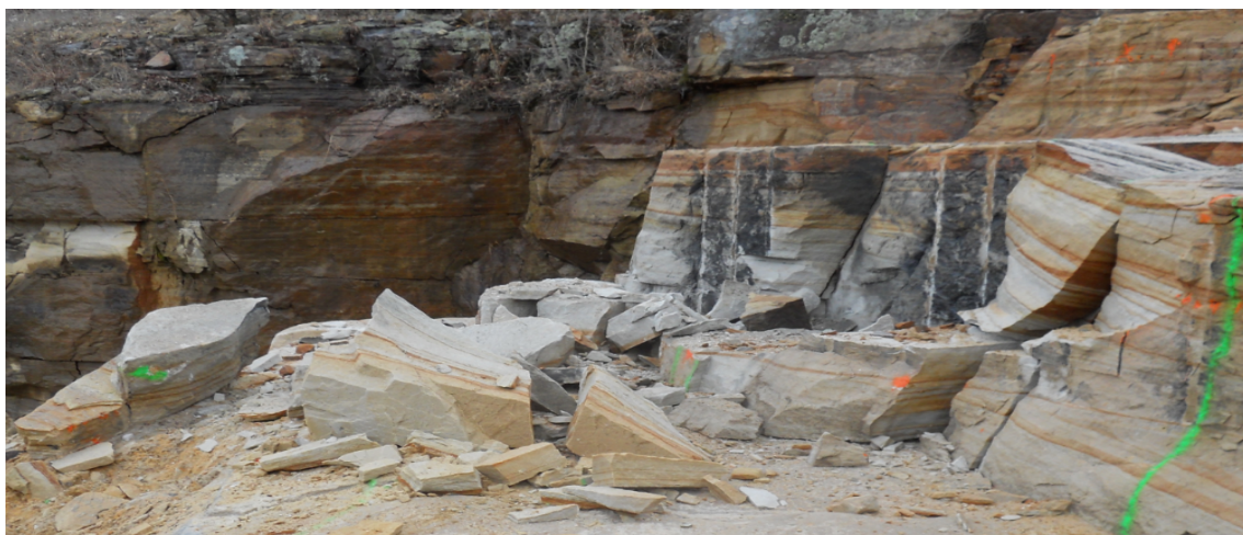
Figure 4.5: Fractures present in the shot area caused some of the stone to break into small rocks during the blast and had to be regarded as waste.
