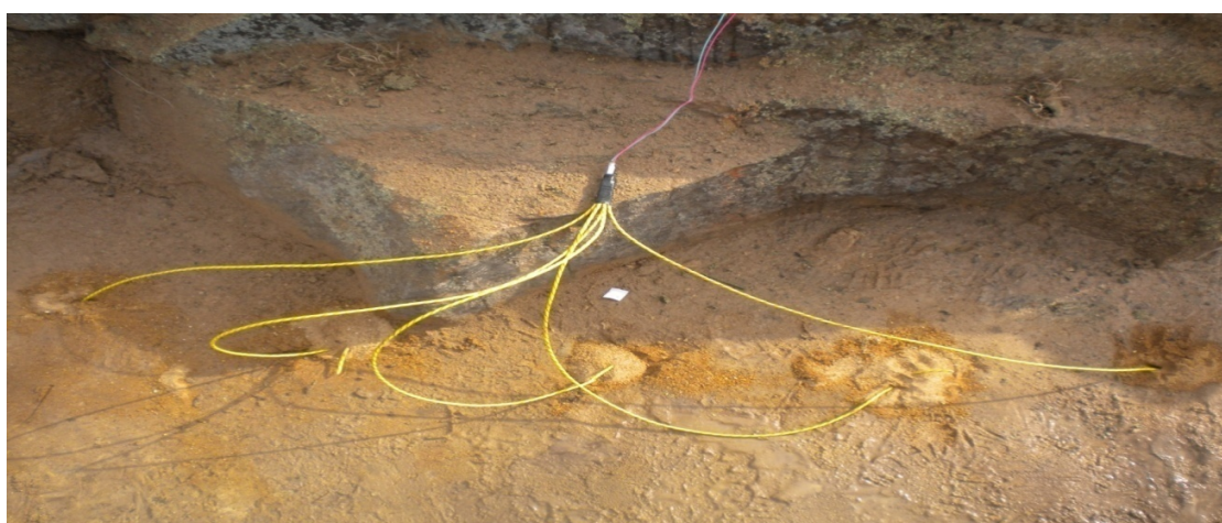
Figure 5.9: Five equal lengths of donor cord connected to one electric detonator.
