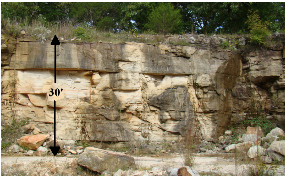
Figure 4.3: The high-wall produced by DiPardo's excavation methods shows a cross section of the sandstone being mined at the quarry.
