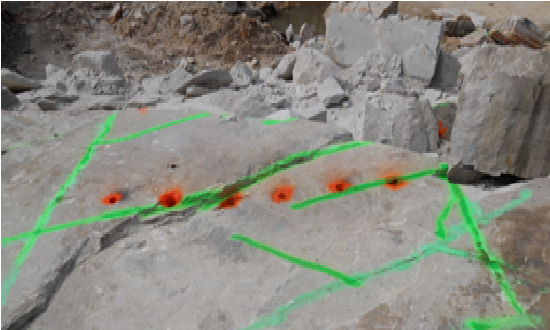
Figure 5.2: After drilling, the final burden for each hole was documented, and the natural seams and joint sets were marked with green paint.
