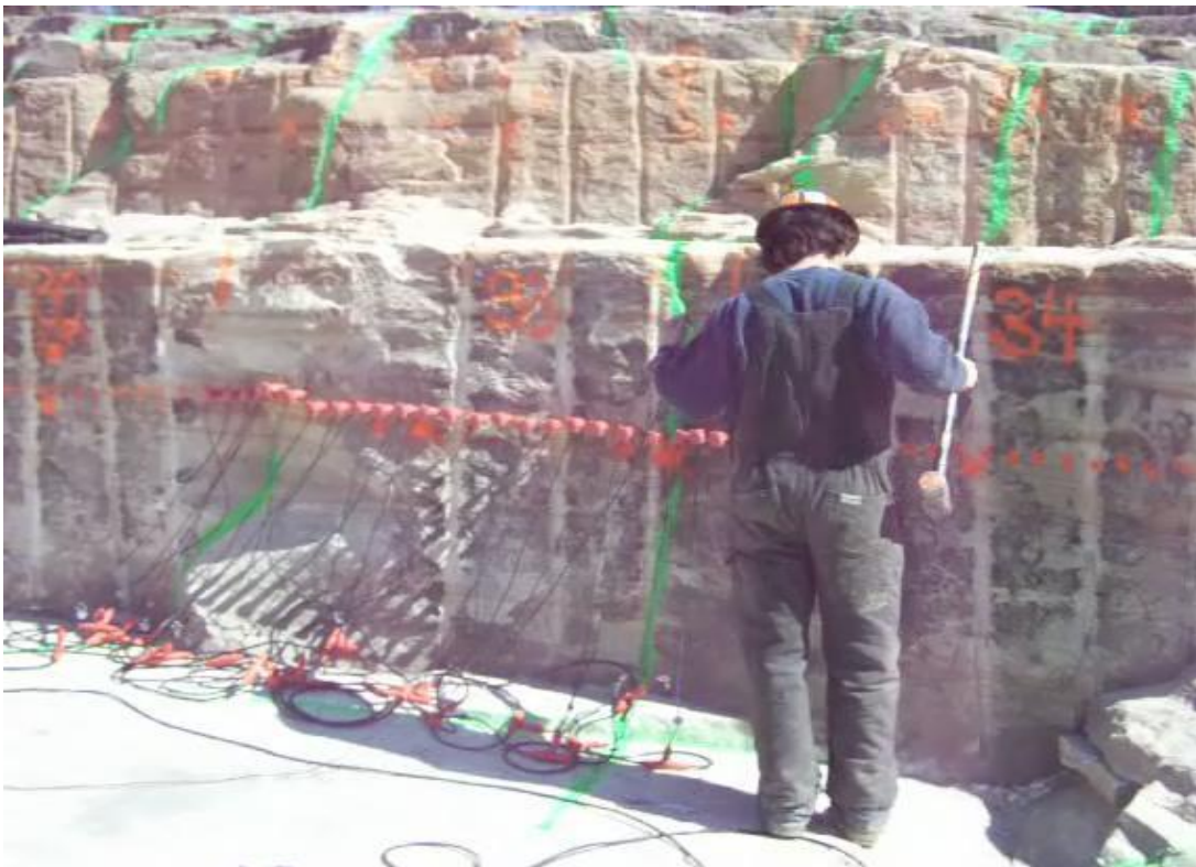
Figure 5.12: A 4.5 kilogram (10 lb.) sledge hammer was used as the impact source on the rock face where the geophones were embedded into the stone.
